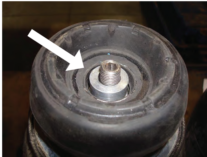
Rubber removed from VR6 mount
