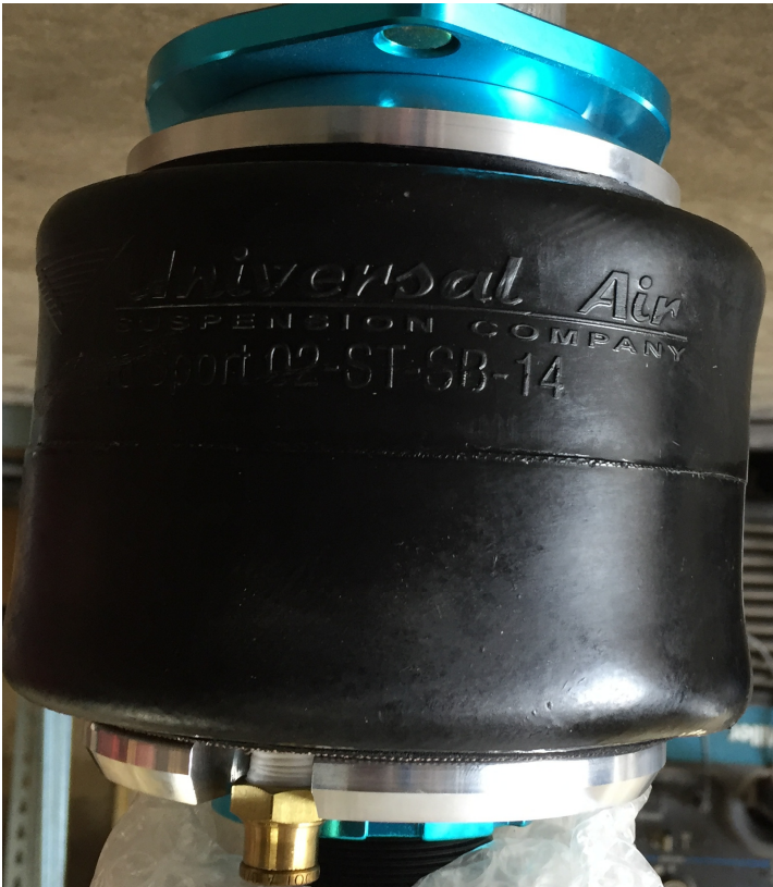
This Bag is adjusted properly. Bellows are flush with upper/lower caps
