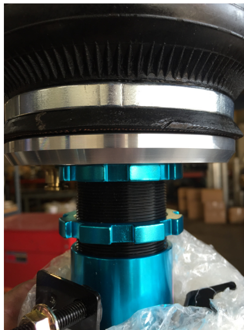
15. Loosen lower lock ring and install strut on car. Fully compress the suspension and look at how it sits.
