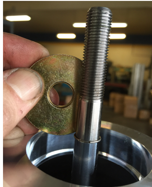
12. Install washer with groove facing downwards to the wire on the shock shaft
