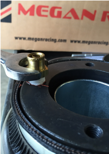
9. Install Air Fittings into the Bags. Hand tight and 1 turn with a wrench. DON'T OVER TIGHTEN!
