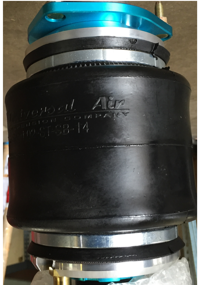
This Bag is not fully compressed. Bellow isn't flush with caps of the bag.
