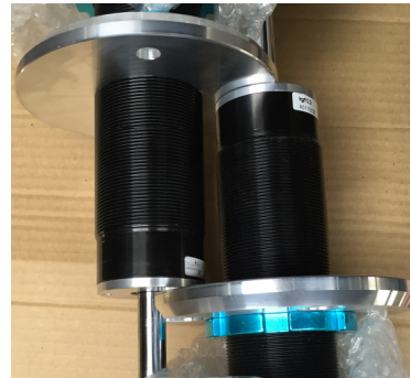
8. After 1 side is set perfectly, invert the other side and match the distance from the bag plate to the top of the shock body to insure both sides are the same
