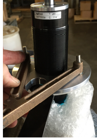
7. Lock down the lower spring perch to lower threaded bag mount.
